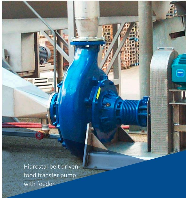
Hidrostral belt driven food transfer pump with feeder.
