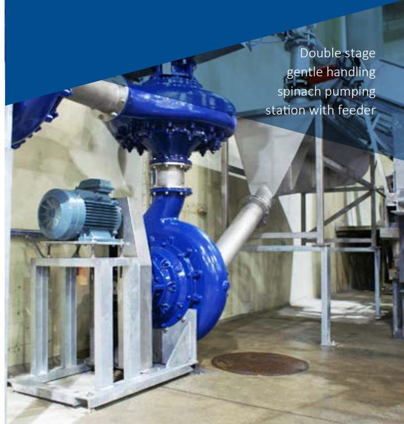
Double stage gentle handling spinach pumping station with feeder
